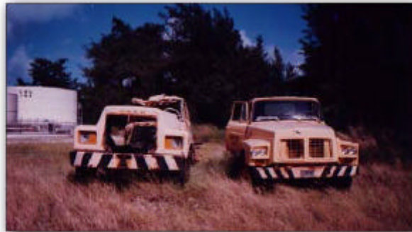
The Mack truck tractor (left) is shown without an engine, transmission, and radiator.
